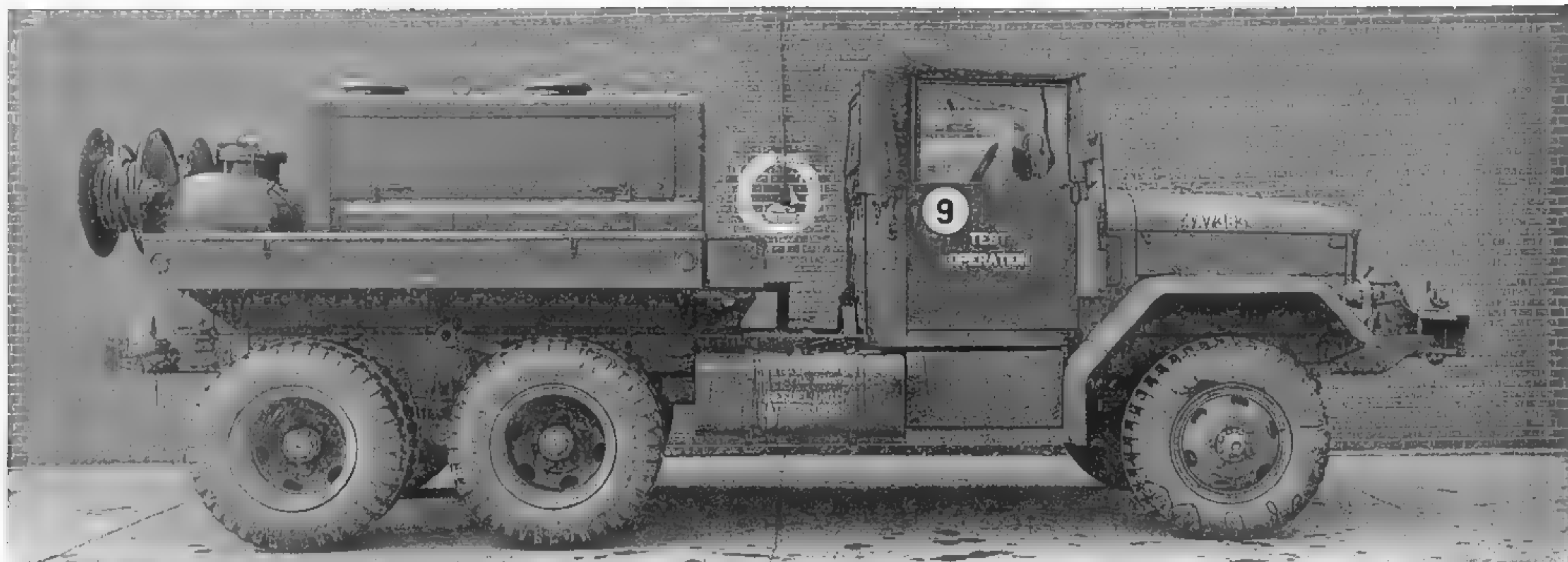
Here is the Davey 210 WDS. Like the Le Roi, its capacity was 210 cu. ft. of compressed air per minute. (Photo courtesy of the Patton Museum)
